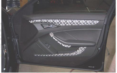
disconnect the light at the bottom of the door. After removing the door panel you will be able to remove the door catch by removing the speaker.
