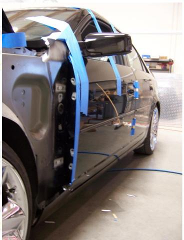
Insert spacers after removing the factory hinges. Hint\*(You can make your spacers out of paint sticks and about 8-10 turns of blue painters' tape)
