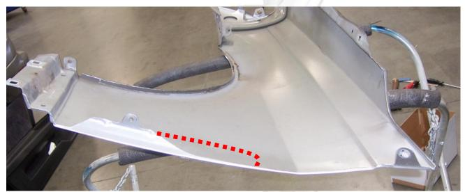
NOTE: The idea of cutting the fender is to give the VDI kit room to move freely the cut out on your car may be different.
