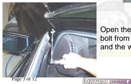
Open the door and remove (1) 10mm bolt from the top, between the door and the windshield pillar.
